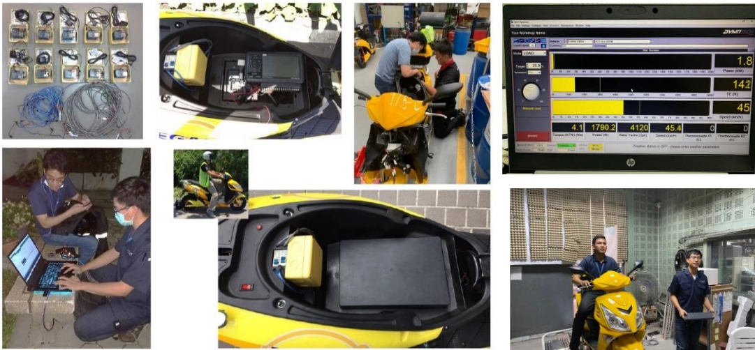
Building and installation photos with 11 EGAT E-Bike; Electric motorcycle on chassis dynamometer; Captured screen of the dynamometer monitoring program
